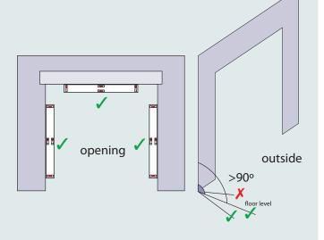
The threshold must be flat/level and sound across the full width of the opening.
